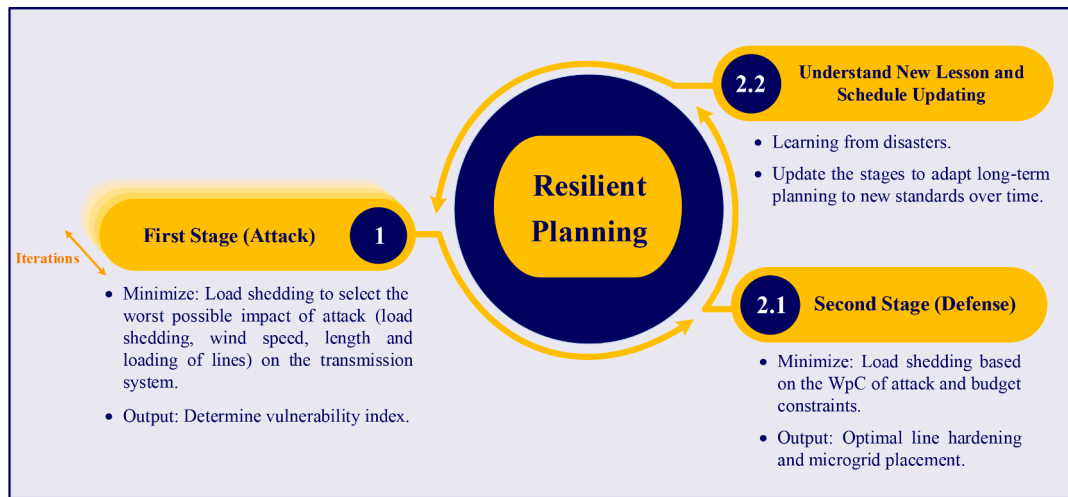
Fig. 6. The linear two-stage optimization problem based on the AD-RP model.
